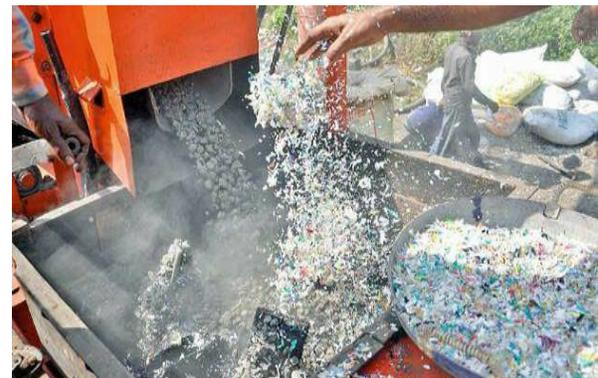
molten Plastic with Stone and bitumen, a black tarry substance, used to lay roads, he observed, it bound together and improved the tensile strength of road, making it more durable and flexible. Also , using plastic as a binder , the quantity of bitumen utilized was reduced by 6-8%.
